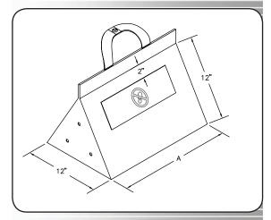
The Dock Stufr® easily and inexpensively eliminates dock gaps. Simply toss the Dock Stufr into place during the loading process. Its flexible and compact size fills in gaps yet does not interfere with loading.
