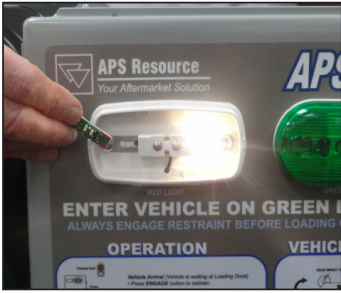
Inside LED Upgrade
