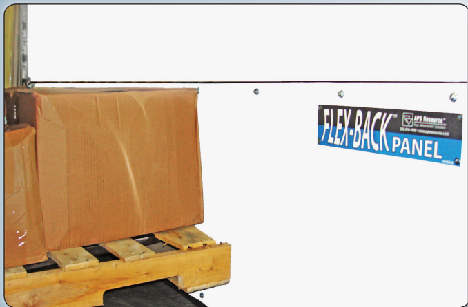
FLEX-BACK Door Panel Flexes Upon Impact
