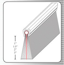
The WeatherWall is a unique style of brush weatherseal. The WeatherWall has a sheet of EPDM rubber surrounded by a layer of brush on each side. You get the benefits of brush seal with the air stopping feature of a EPDM rubber seal.
