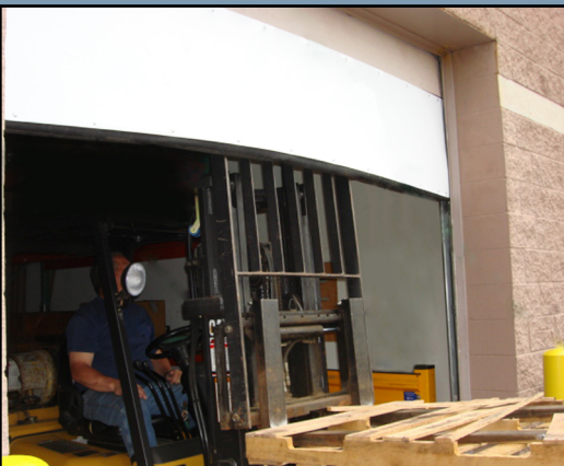
Figure 2: The panel flexes on impact but returns to normal operating position
