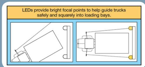
Figure 2: Top view diagram
